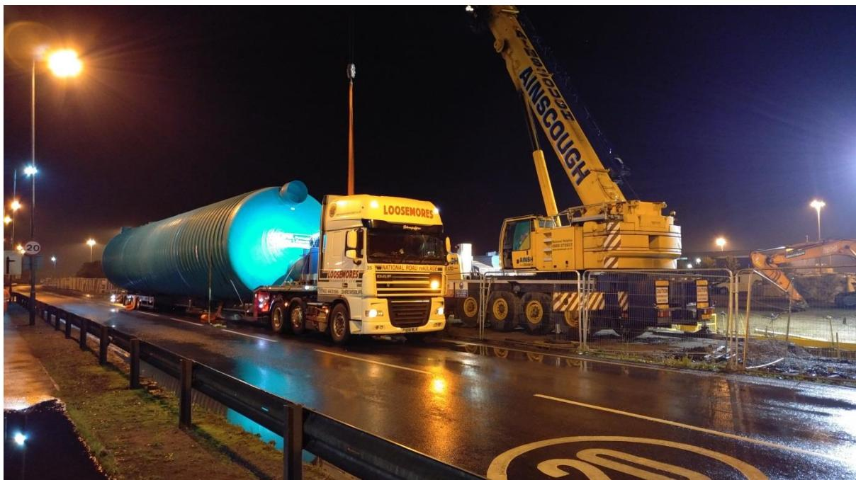
At 8pm on Thursday 21st September 2017, CRO Ports at North Killingholme, Immingham in South Humberside, closed its busy road to receive the SPEL P800/1CSC Puraceptor® Class 1 full retention separator - 4.15m in diameter and 25m long (approximately 300,000 litres) and was delivered as
